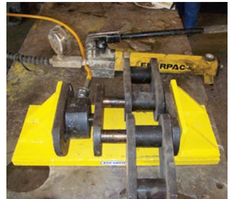
The PCA Innovation in Safety Award winning entry. Shown is the jig and hydraulic press in place ready to press on a side plate.
